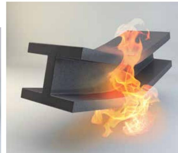
At a critical temperature of 500°C steel loses its strength. Fire resistance ratings are only far less than 30 minutes.
