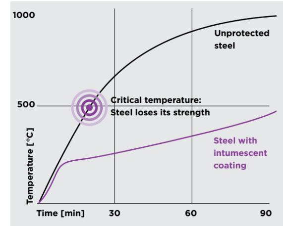
Temperature of steel over time in a typical fire with and without intumescent coating.
